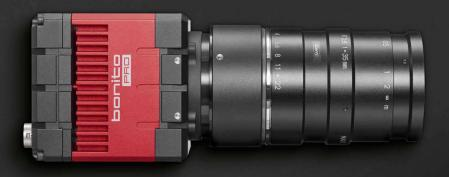
Bonito PRO is Allied Vision's high-bandwidth camera series with a CoaXPress interface. Equipped with four DIN 1.0/2.3 connectors, the camera is capable of transmitting 25 Gbps via four CXP-6 high-speed connections. Bonito PRO boasts a rugged, fan-less housing design and powerful feature set – making it the ideal choice for high-definition imaging applications that require high throughput, robustness, and system design-in flexibility.
